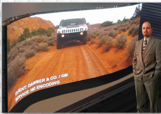
TR2006R curved 24 modules arranged 8 wide by 3 high. 3077mm (10.08 ft) by 1152mm (3.79 ft)
